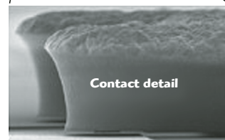
▲ Fig. 2 SEM photographs of the Radant MEMS switch package (a) the actuator (b) with detail of the contact area (c).
